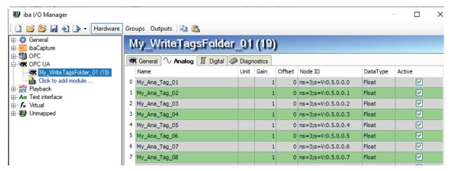
If required, you can change the signal names afterwards in the signal tables in the OPC UA server module. This has no effect on the tag names.
